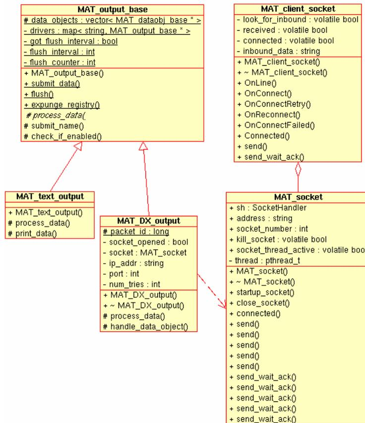
Figure 24 – UML Diagram of the DCIL Output Interface Classes
