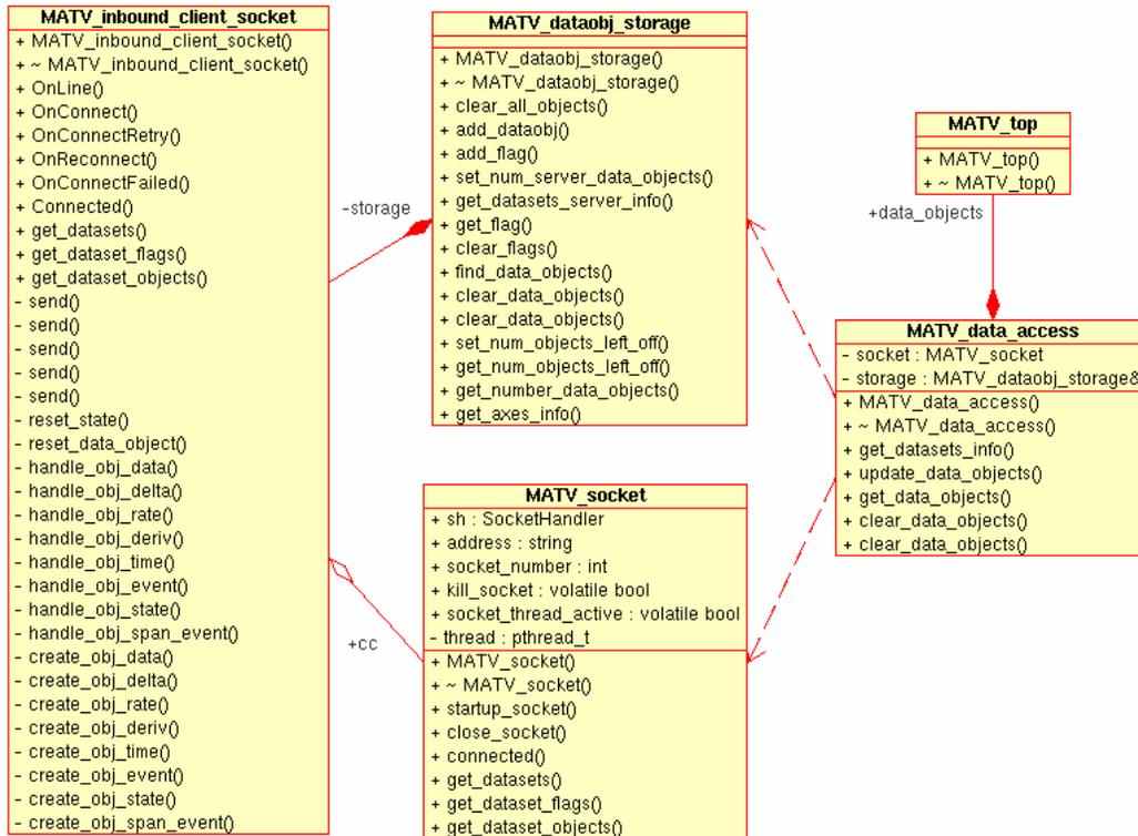
Figure 26 – UML Diagram of the *MATView* Inbound Interface Classes
