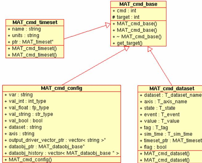
Figure 18 – UML Diagram of the DCIL Command Classes
