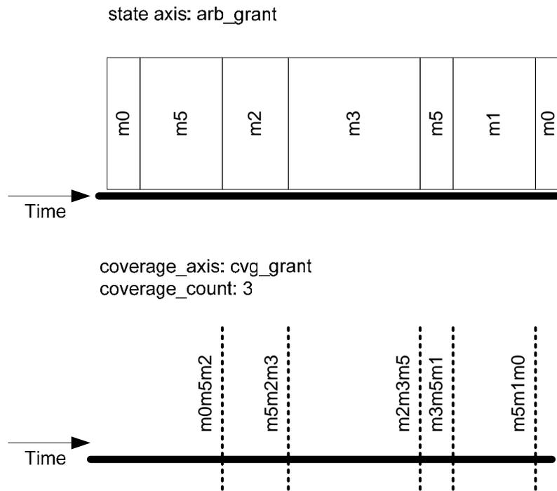
Figure 16 – Example State Axis and Auto-generated Coverage Axis
