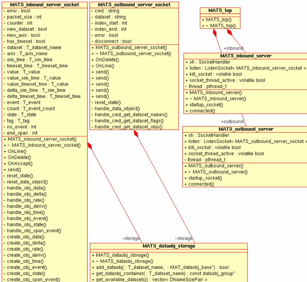
Figure 25 – UML Diagram of the *MATSrv* Classes
