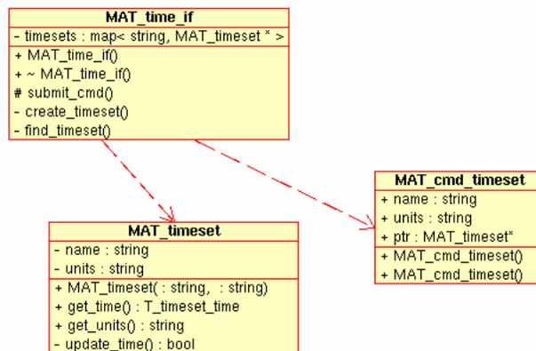
Figure 22 – UML Diagram of the DCIL Timeset Execution Unit and Related Classes
