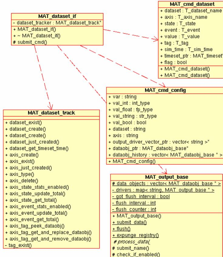
Figure 21 – UML Diagram of the DCIL Dataset Execution Unit and Related Classes
