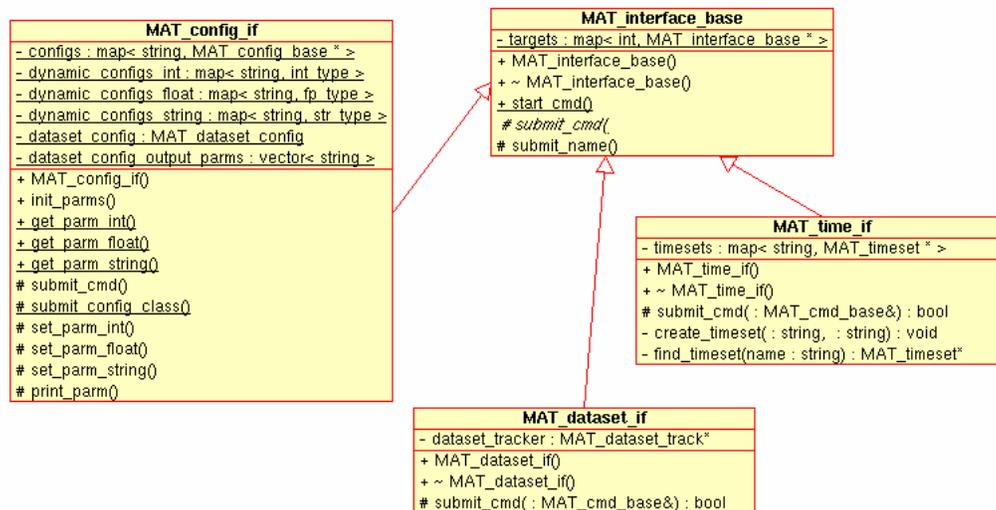
Figure 20 – UML Diagram of the DCIL Command Bridge Classes
