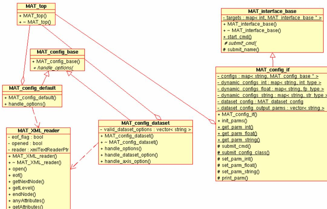
Figure 19 – UML Diagram of DCIL Configuration Classes
